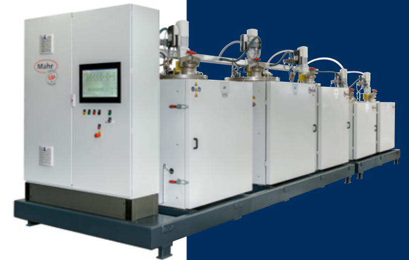
MarMax CS 60 PUR Elastomer machine
