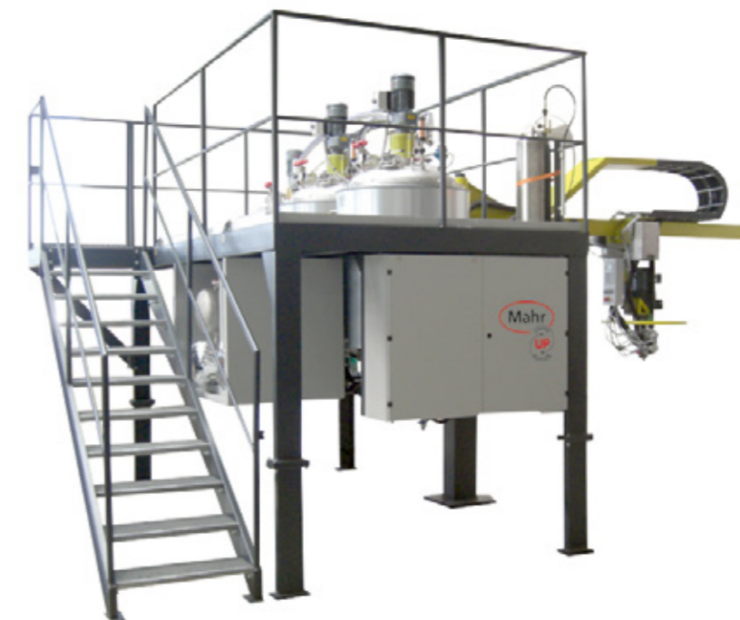
Accessible 3 component PUR-Hot casting machine
